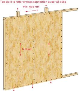
Bottom plate to floor or sub floor connection as per AS 1684
