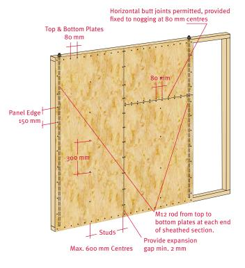
Note: For all above systems, minimum joint strength of framing JD5. No noggings required for full height sheets unless being used for internal wall bracing, see page 10. **Min. 2 mm expansion gap around perimeter of panel.**
